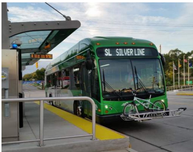
Level boarding for customers at an enhanced transit stop in Grand Rapids, Michigan
