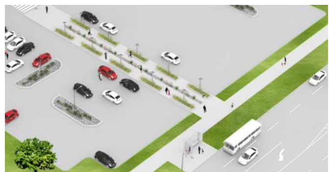
A clear pedestrian pathway connects the building entrance to a transit stop
