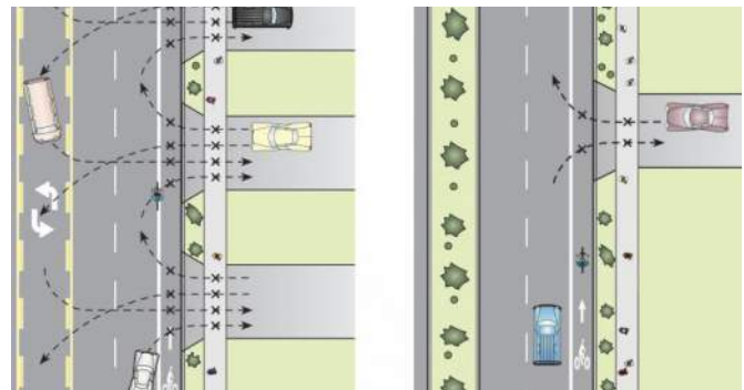
Conflicts with multiple driveways (left) Reduced conflicts with consolidated driveways (right) Source: www.ahtd.info
