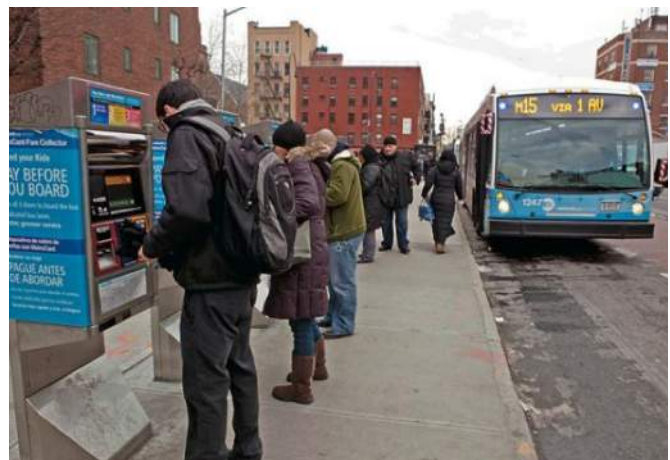
Riders pay their fare prior to boarding the bus helping to reduce dwell time at a stop Source: www.untappedcities.com
